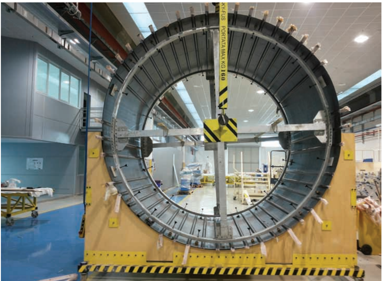
Alenia Aermacchi composite fuselage One Piece Barrel (OPB) demonstrator. It leads to weight reduction due to more innovative multi-functional layer and multi-layer architectures, better acoustic insulation and increased hail impact performance.
